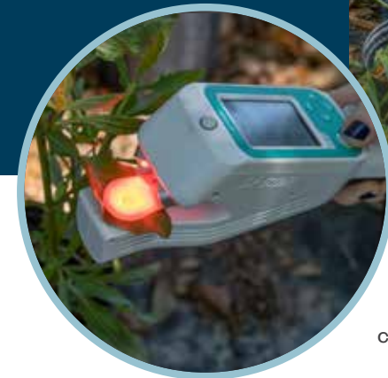
Ecology student Mary Moody uses an instrument that measures photosynthesis and levels of stress in plants. Photos by John Eder
